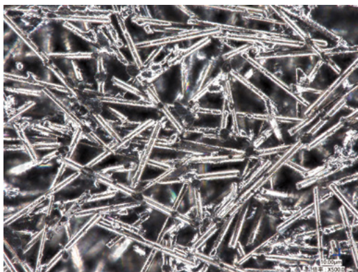
ガス拡散層の拡大写真(×500倍) / Enlarged photo of gas-flow channels (×500)
