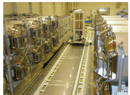
バッチ式真空加熱乾燥装置 Batch-style vacuum heating and drying furnaces
