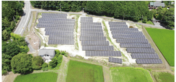
太陽光発電のピークカット電力の利用で瞬停防止、電圧変動を安定させる Prevents instantaneous power failure and stabilizes voltage fluctuation by utilizing peak-cut electricity from solar power generation
